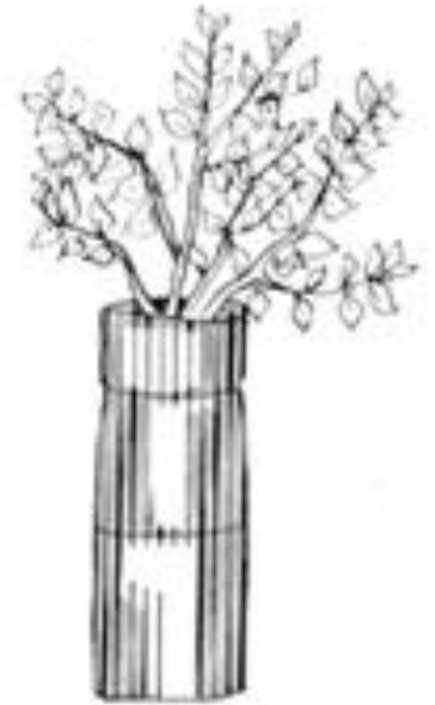
Insulative wrap (aluminum foil backing or fiberglass).
